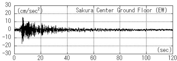
Figure 2.13 Observed Acc. on the Ground FL (EW)
