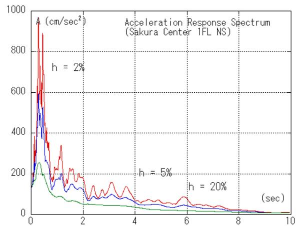
Figure 2.4 Acceleration Response Spectrum (NS)
