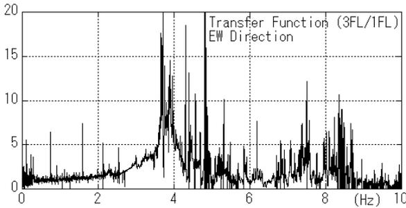
Figure 2.21 Amplitude Transfer function of 3<sup>rd</sup> FL/GL (EW)
