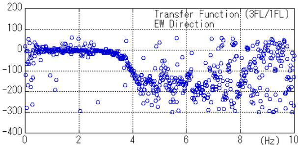
Figure 2.23 Phase transfer function of 3<sup>rd</sup> FL/GL (EW)
