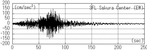
**Figure 2.7 Observed Acc. On the 3<sup>rd</sup> FL (EW)**
