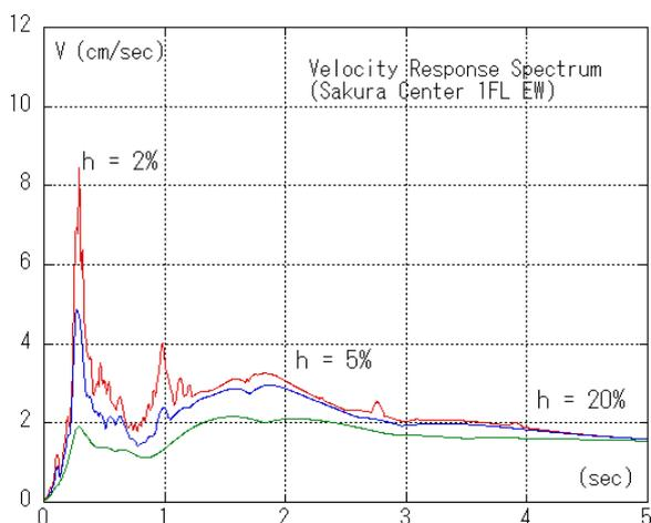
Figure 2.17 Velocity Response Spectrum (EW)
