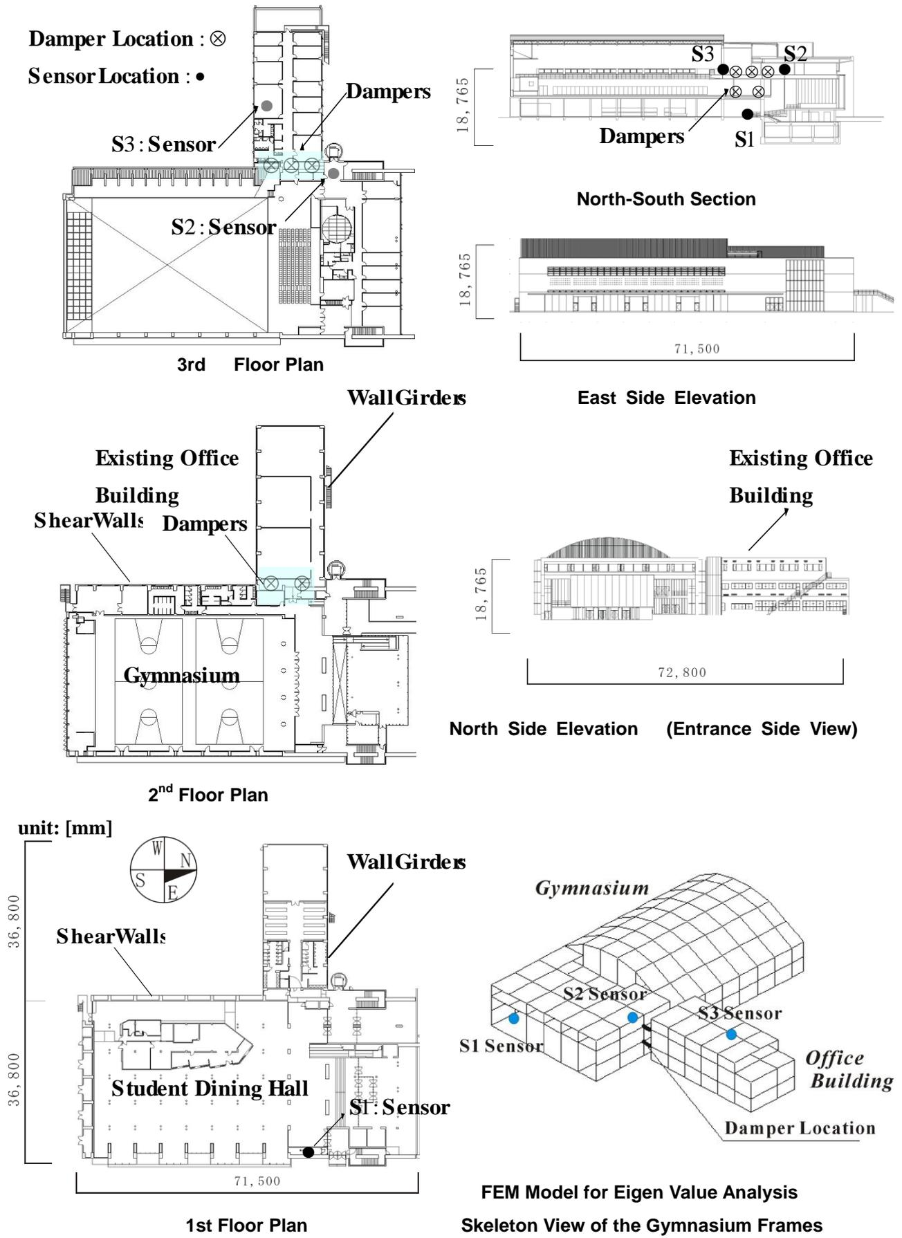
Figure 1.1 Sensor Locations and Damper Locations
