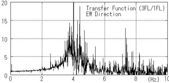
**Figure 2.9 Amplitude transfer function of the 3<sup>rd</sup> FL from Ground FL (EW)**
