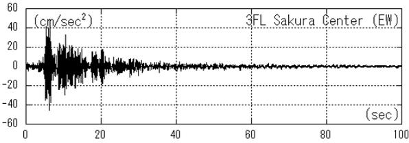
Figure 2.19 Observed Acc. on the 3<sup>rd</sup> FL (EW)
