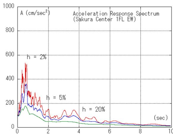
Figure 2.3 Acceleration Response Spectrum (EW)
