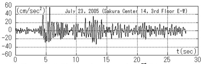
**Figure 1.8 Observed Acc. on the 3<sup>rd</sup> FL**
