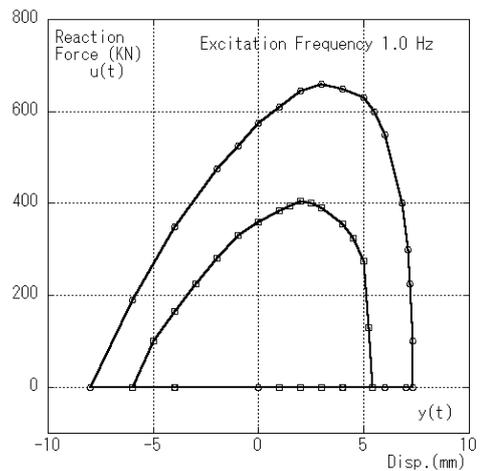
**Figure 1.4** Cyclic loading test results
