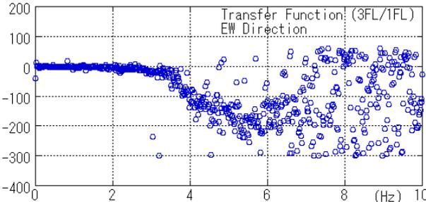
**Figure 2.11 Phase transfer function of the 3<sup>rd</sup> FL from Ground FL (EW)**
