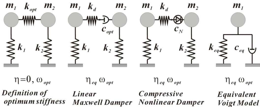
**Figure 1.2** Mathematical model for the nonlinear damper devices in EW direction
