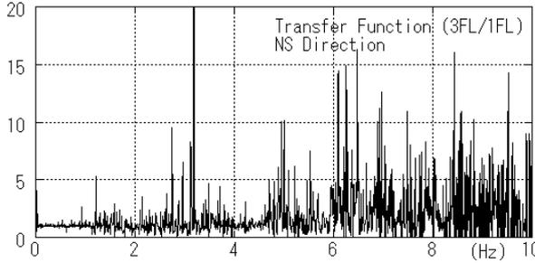
**Figure 2.10 Amplitude transfer function of the 3<sup>rd</sup> FL from Ground FL (NS)**
