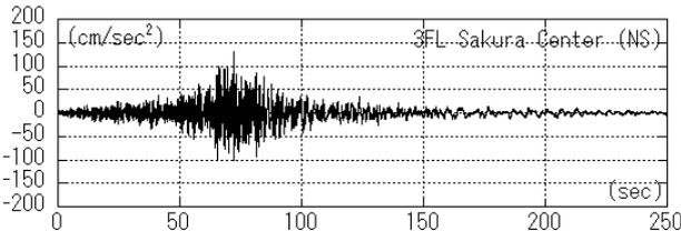
**Figure 2.8 Observed Acc. On the 3<sup>rd</sup> FL (NS)**
