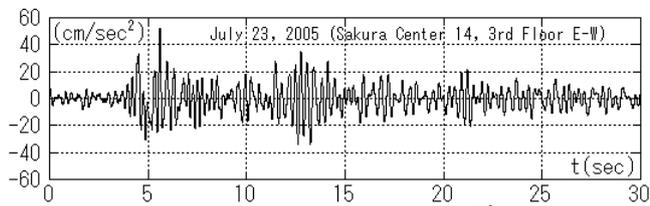
**Figure 1.10 Simulated Acc. on the 3<sup>rd</sup> FL**
