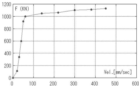
**Figure 1.3** Test results of damper coefficient
