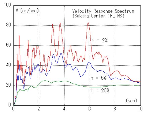
Figure 2.6 Velocity Response Spectrum (NS)
