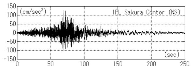
Figure 2.2 Observed Acc. on the Ground FL (NS)
