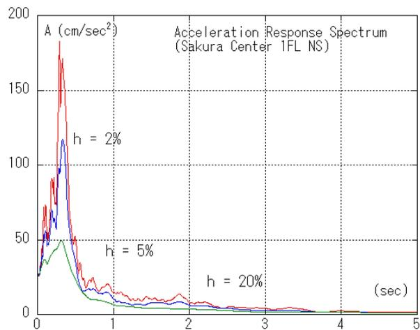
Figure 2.16 Acceleration Response Spectrum (NS)
