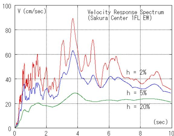
Figure 2.5 Velocity Response Spectrum (EW)
