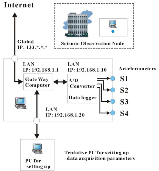
**Figure 1.7 Local network sensor system**
