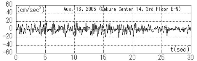
**Figure 1.11 Simulated Acc. on the 3<sup>rd</sup> FL**
