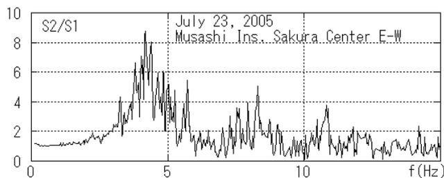
**Figure 1.14 Transfer Function (3FL/GL)**
