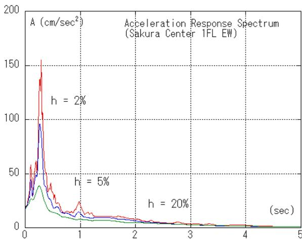
Figure 2.15 Acceleration Response Spectrum (EW)
