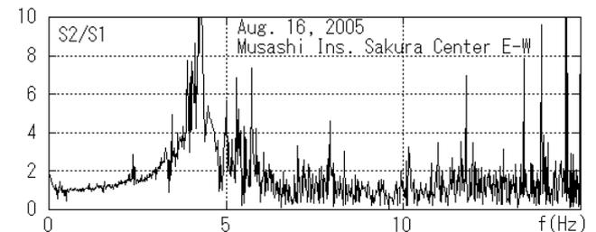
**Figure 1.15 Transfer Function (3FL/GL)**
