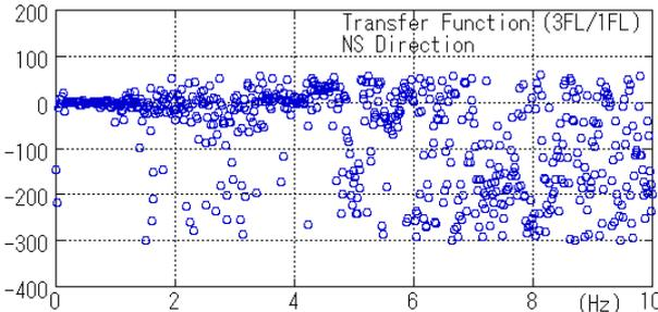
**Figure 2.12 Phase transfer function of the 3<sup>rd</sup> FL from Ground FL (NS)**
