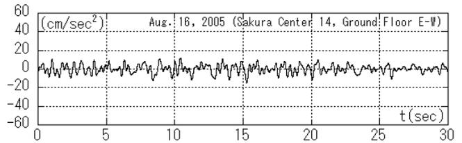
**Figure 1.13 Observed Acc. on the Ground FL**
