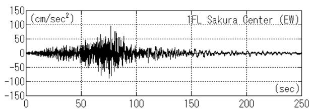
Figure 2.1 Observed Acc. on the Ground FL (EW)
