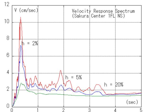
Figure 2.18 Velocity Response Spectrum (NS)
