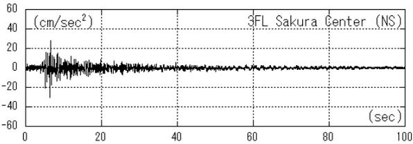
Figure 2.20 Observed Acc. on the 3<sup>rd</sup> FL (NS)
